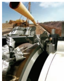
Formed tool bits for wall thicknesses in excess of 2.5in.
