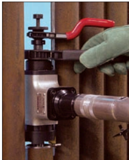
The "Tube Weasel" fits a Dutchman window for single tube end prep work and totally sealed construction allows it to be used in any orientation. Most importantly, the holding clamps are designed to stay on the mandrel and not fall down the tubes.
