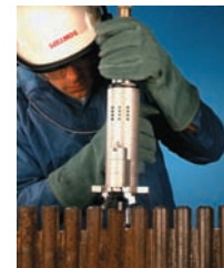
Both the HHB-5,000 and HHB-10,000 Straight Drive models can be hand held or track mounted.
