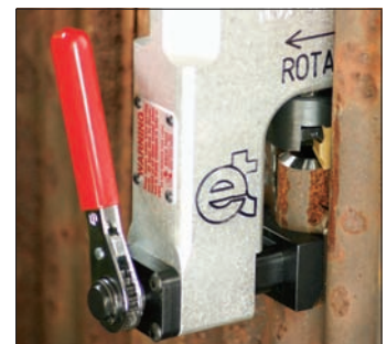
This rugged tool has a narrow profile and fits between 1-1/4" O.D. membrane water wall boiler tubes.
