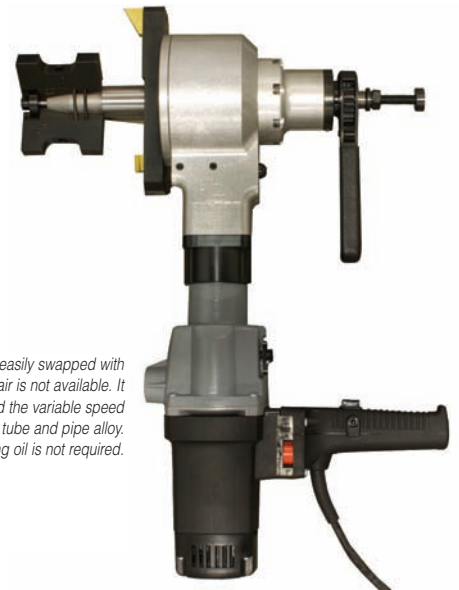
The Prepzilla MILLHOG® cuts heavy wall pipe and tube, producing a heavy chip with no cutting oils; resulting in perfect end preps.
