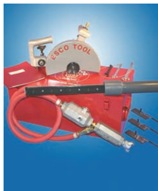
The PANELHOG® APS-438 Air Powered Saw glides along the EscoTrack System for boiler tube panel removal, producing a straight, clean horizontal cut that requires no further rework.
