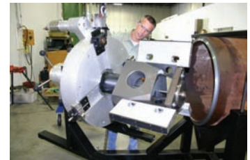
Only eight sets of clamps and two wedges required to cover entire range. Simple to operate, quick to set up.
