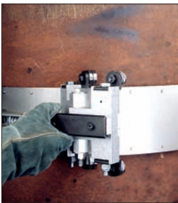
Trolley is adjustable for a variety of EscoWrap Tracks
